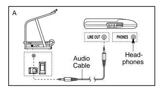
B. Plug one end of the audio cable into the jack on the side of the hiker near the power cord. Plug the other end of the cable into a 3.5mm Y-adapter (available at electronics stores). Plug the Y-adapter into the PHONES jack on your CD player. Plug your headphones into the other side of the Y-adapter.
